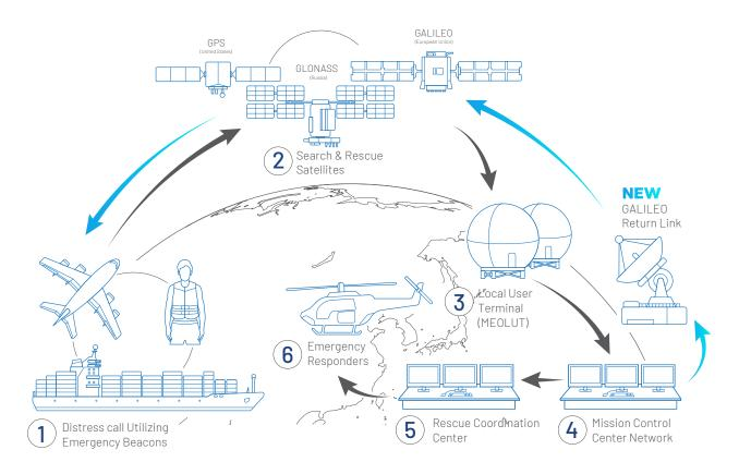
beacon to inform the user that their distress signal and location have been detected. This new capability is unique to the Galileo satellites and was activated in January 2020 and declared globally operational by Cospas Sarsat in March 2021. The world's first RLS enabled PLB, the FastFind Return Link has been available to buy since March 2021.
