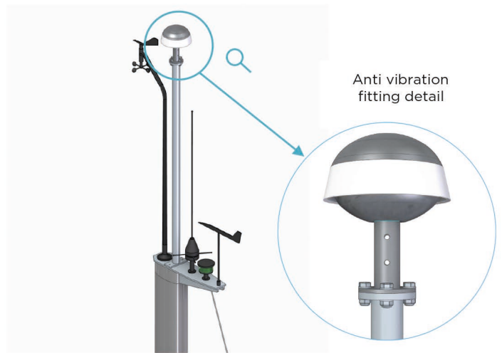
Figure 8. Standard mast installation.
