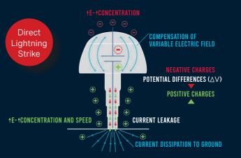
The idea of conventional lightning protection is to attract the lightning and to discharge it on a controlled path to the water. But the difference between yachts and houses are the small distances on yachts. The result is that lightning strikes typically damage the electronics due to induced overvoltages on yachts. Also, the mast needs to be replaced after a strike very often.
